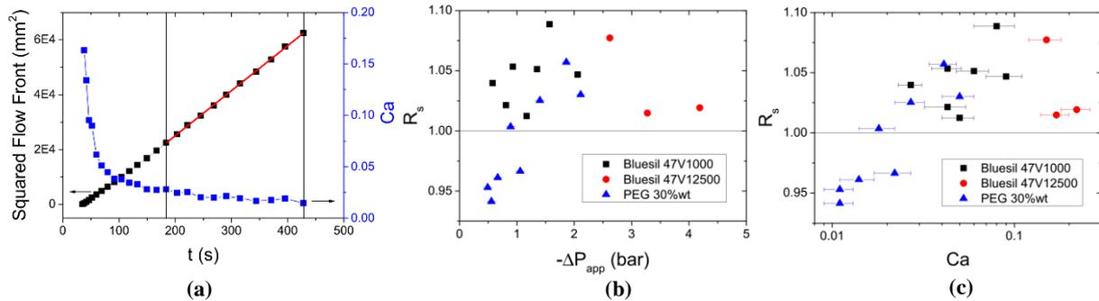
**Figure 1:** (a) Squared flow front and capillary number against time for the experiment with Bluesil™ 47V1000 at 0.46 bar. (b) Ratio  $R_s$  for all the experiments as a function of the applied pressure difference. (c) Ratio  $R_s$  as a function of the average capillary number for all the experiments.
